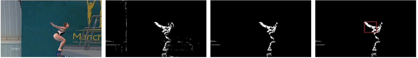
Fig. 3. Selection of the MSR in the human body. Left to right: Input RGB image, extracted MSR candidates, small MSR candidates discarded, and the most salient motion region.
